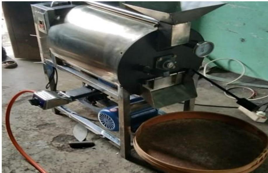
Gambar 1. Contoh Mesin Roasting Kopi bahan logam stainless steel
